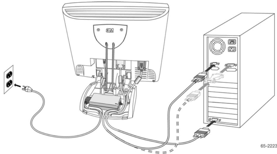
You should be sure all cable connections are secure -- tighten all cable screws. Shaking and vibration may dislodge cables that are improperly connected.
