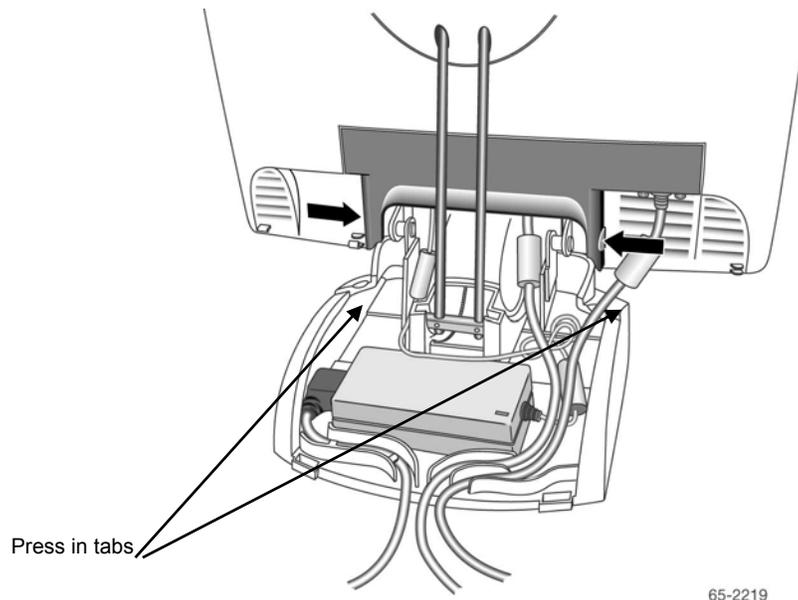
4. Push in on the cable connector tabs as shown above to release from display back. Gently pull down to release tabs.
