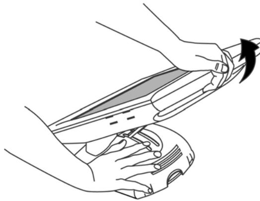
Lift up on the latch to release lock. Adjust the M1700SS Display by pushing or pulling on the top front of the display until the screen is at the best viewing angle for you. Then push down on latch to engage locking mechanism and stabilize display position.
