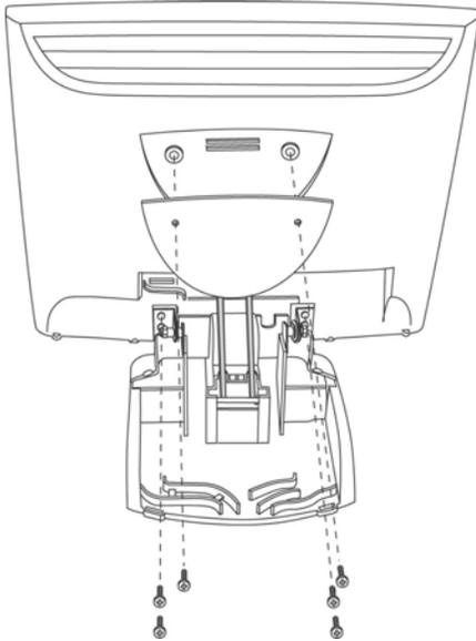
Step 1 – Unlock front mechanism and disconnect all cables from the display.
