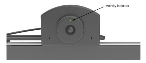
Step 5. Start your conferencing software and enable the camera. The green activity indicator will illuminate any time the webcam is in use.
