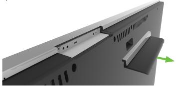
**Step 2**. Plug the conference camera into the Elo Edge Connect<sup>™</sup> dock ensuring the USB connector on the camera aligns with the matching connector on the IDS display. Install the two M3 mounting screws to secure the camera to the IDS display.
