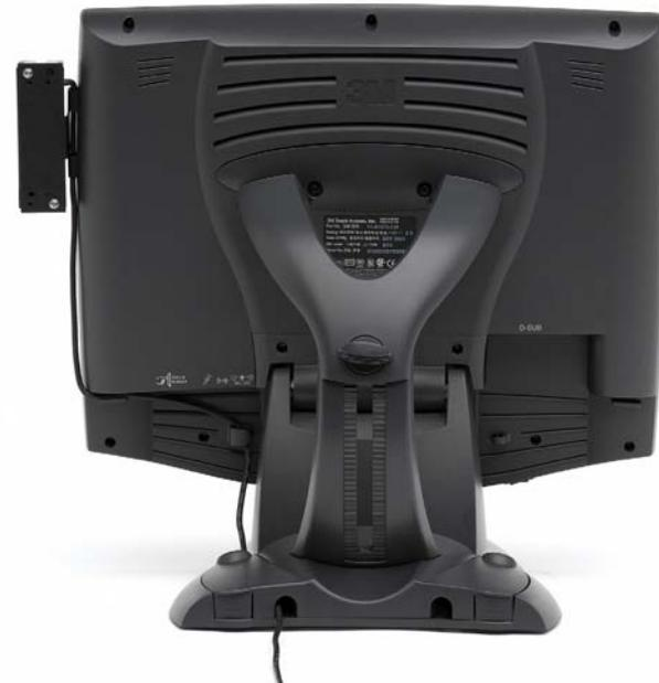
Attachment plate mounts on left or right side of monitor
