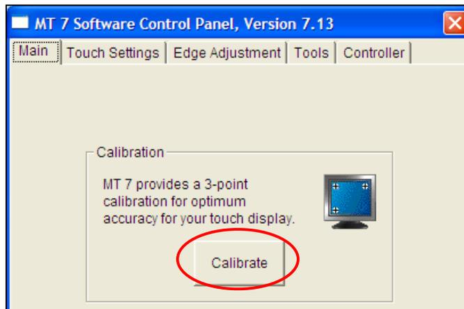
2. You may calibrate by accessing the Software Diagnostic Utility (SDU) found on the enclosed CD.
